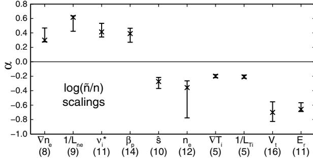
**Figure 4.** 10th–90th percentile ranges for scalings that emerge from model aggregation for  $\log(\delta n/n)$ .  $\alpha > 0$  ( $\alpha < 0$ ) denotes a positive (negative) scaling, and numbers below labels indicate the number of models that contain the scaling.
