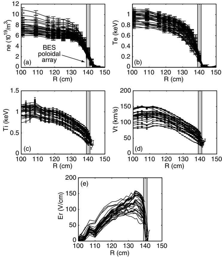
**Figure 1.** A subset of plasma profiles in a database for ELM-free, MHD-quietest phases in H-mode plasmas. The grey box denotes the BES poloidal array at  $R = 140$  cm.
