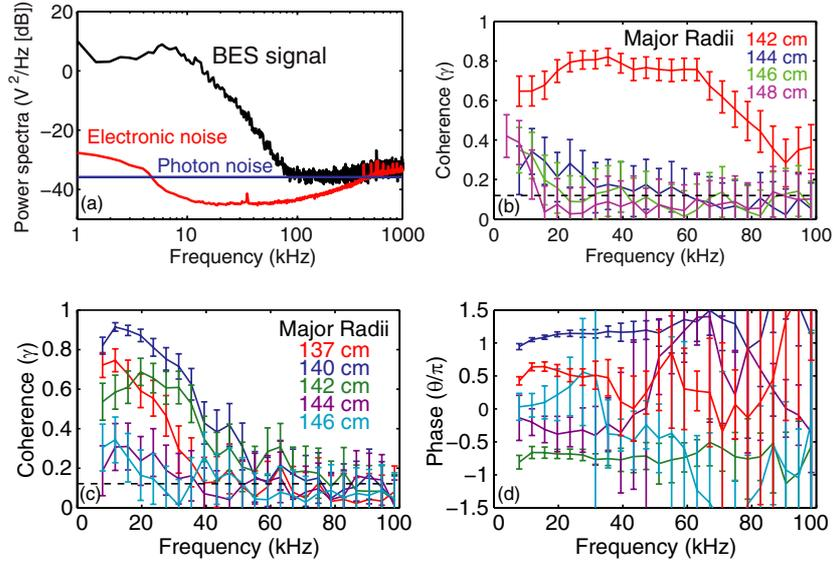
**Figure 2.** (a) Power spectra for BES signal, electronic noise, and photon noise. (b) Coherence spectra for radial channels outboard of the measurement location at  $R = 140$  cm. (c) Coherence and (d) cross-phase spectra for radial channels spanning the pedestal relative to the core channel at  $R = 129$  cm. The dashed line in (b) and (c) represents the coherence noise level.
