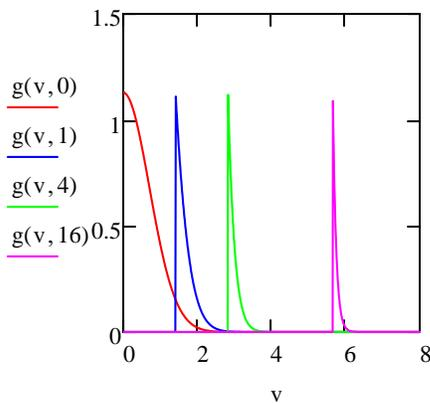
As our electron beam accelerates, the minimum velocity determined by the potential drop determines the velocity where the distribution function begins.
