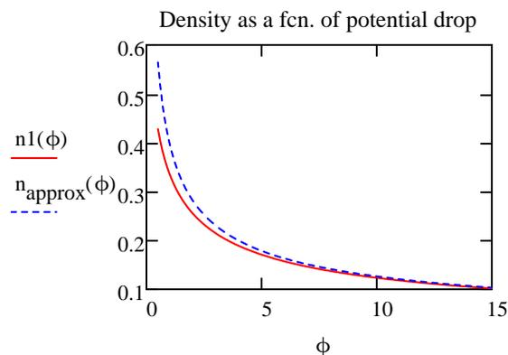
This plot compares two ways of finding the density.  $n1$  uses Liouville's equation and is exact.  $n_{\text{approx}}$  uses the continuity equation, and divides the current by the approximate velocity to obtain the density.
